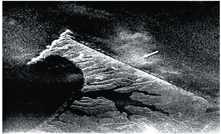
Figure 3. Example of space-based radar image showing Point Reyes, CA, 1964. The arrows point to dense rain squalls where visibility was less than ¼ mile. (Source: NRO experimental Quill program; courtesy of CSNR Reference Collection as published by CSNR in Trailblazer 1964: The Quill Experimental Radar Imagery Satellite Compendium , edited by J. Outzen.)
