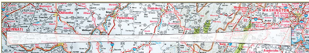
Figure 23. Graphic depiction of the ground area in a single Hexagon KH-9 panoramic camera frame for its coverage of the 370 nautical miles between Cincinnati, OH and Washington, DC (Source: CSNR Reference Collection)
